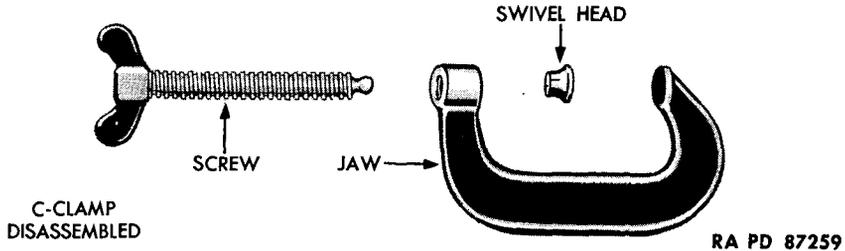
2. Using new parts as needed, turn the screw into position through its boss at end of jaw. Slip swivel head onto ball on end of screw and crimp head sufficiently to hold it on ball.
