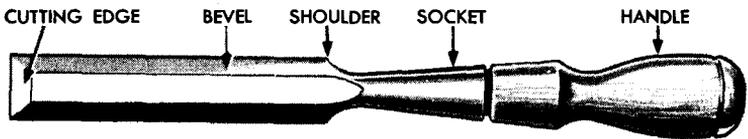
WOODWORKER'S CHISEL (BEVEL EDGE BLADE)
