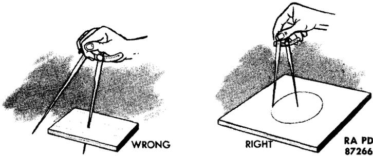
Do not lay dividers on bench when not in use. They may be damaged by other tools. Keep them in case or wrapped in cloth and stored in a safe place.
