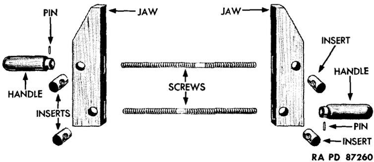
2. Using new parts as necessary, place inserts (if any) in position in jaws. Turn both screws into position in the two jaws. Install handles on screws.
