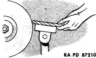
4. Slowly place heel of drill against grinding wheel. Then gradually raise shank end of drill and twist drill in fingers in a counterclockwise direction while grinding wheel approaches the cutting edge. Exert only enough pressure to grind the drill without overheating. Frequently cool drill in water while grinding.
