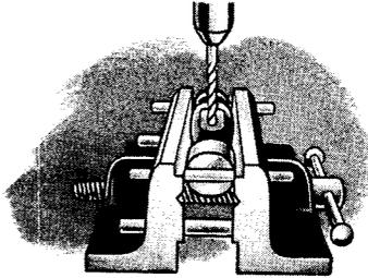
3. Drive old handle from head and secure wedges. (Note position of wedges.)
