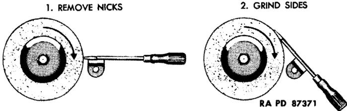
2. Adjust rest to hold screwdriver against wheel to give desired parallel or concave shape. Grind both sides until tip is of required thickness.
