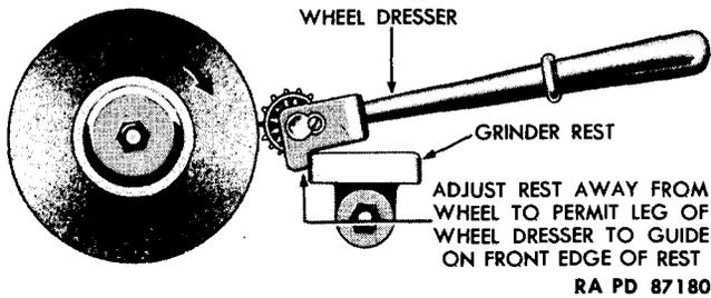
1. Adjust tool rest to permit wheel dresser to contact abrasive wheel on centerline of wheel as illustrated.
