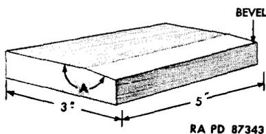
Place saw on block as shown in sketch. Clamp saw and block together. Place a blunt end punch on tooth to be set. Strike punch smartly with a hammer to set tooth. Similarly set every second tooth which is over block. Move block along to set remaining teeth. Apply block to other side of saw to set alternate teeth.
