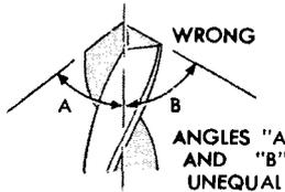
Only one cutting edge will do work. This results in rapid drill wear and causes hole to be larger than drill.
