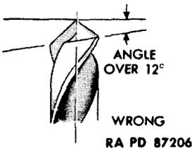
Cutting edges likely to break down due to excessive bite with insufficient support.
