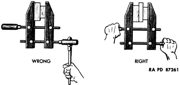
Do not cock clamp to tighten. This procedure may warp, bend, or break clamps. Keep jaws parallel.
