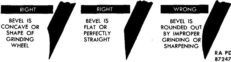
2. Bevel should be about twice the thickness of chisel near cutting edge.
