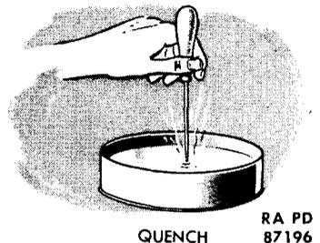
Quickly rub hardened end with aluminum oxide abrasive cloth or oilstone to brighten it. Watch color return to tip from heated portion of blade and quench when light straw color arrives at point. Polish blade with aluminum oxide abrasive cloth and crocus cloth.
