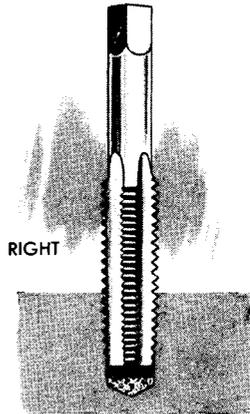
HOLE HAS SUFFICIENT DEPTH TO KEEP CHIPS FROM BINDING
