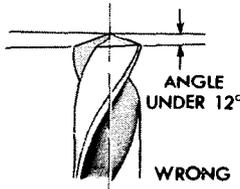
Cutting edges lose effectiveness. Drill won't drill and may split up center when pressure is applied.
