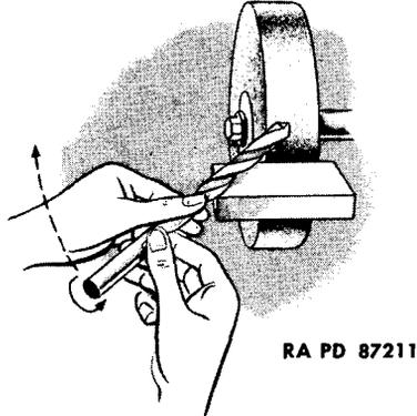
5. Check results of grinding with a gage to determine if cutting edges are same length and at desired angle and if heel is ground to angle of 12 to 15 degrees.
