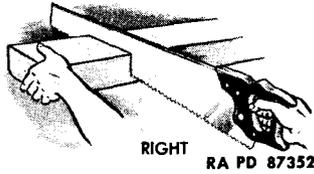
Do not allow end of saw to strike floor. There is danger of springing the blade. Raise work high enough to get clearance. If work cannot be raised, limit the stroke.
