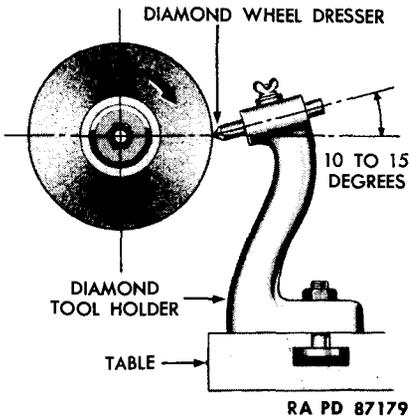
1. Set tool as shown, almost in contact with high point of wheel.
