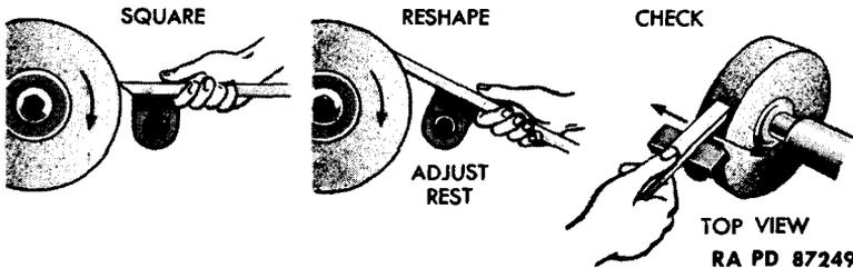
**NOTE:** Special holding fixtures are available. Their use greatly simplifies grinding of chisel type tools.
