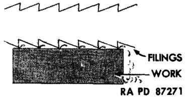
2. Brush filings from between teeth of file with wire brush. Push brush in a direction parallel with teeth.
