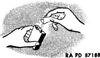
Dust broken edges thickly with flake or ground orange shellac. Carefully work shellac into all cracks and openings.
