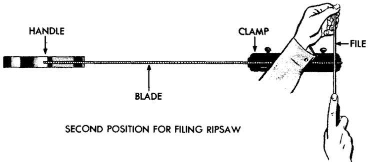
Place file in gullet to *right* of first tooth set toward you. This is the first of gullets you skipped when filing other side of saw. At correct angle (right angle), file until you cut away other half of flat top and teeth are shaped to points. Continue this operation in every second gullet until you reach saw handle. All teeth should be same height and shape.
