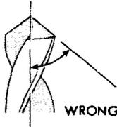
Drills slower and requires more power because of longer length of cutting edges, and requires frequent sharpening.
