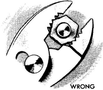
Do not use pliers as a pry bar. Handles may bend or break. Use tools only for purpose for which they are designed.
