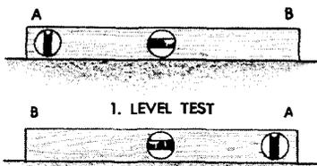
2. Place plumb level against a true vertical surface and note plumb reading. Twist level one-half turn about its vertical axis and again take reading. If bubble appears on opposite sides of hairline in the two readings, plumb level is out of adjustment.
