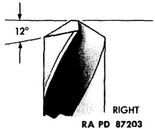
Grind heel to an angle of 12 to 15 degrees (9 degrees for drilling extremely hard material). Failure to provide sufficient clearance is the principal cause of drills splitting up the web.
