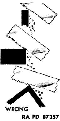
Never start cuts on sharp angles. This practice is likely to strip saw teeth. Start the cut with blade held at a slight angle to the surface.
