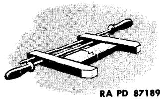
Reheat pieces to melt shellac, and clamp together until cooled. Dress stone if joints are uneven.
