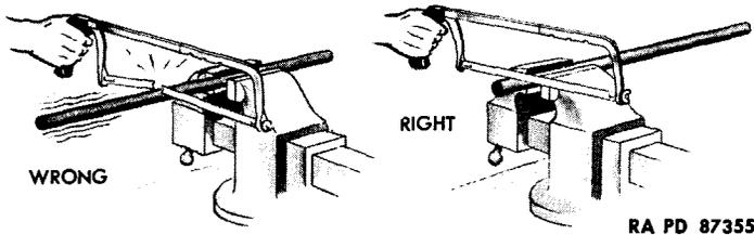
Do not use a new blade in a cut started with another blade. The new blade is likely to wedge and break. Turn work over and start new cut from opposite side.
