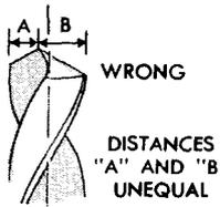
This throws point and lip off center, causing strain on drill, machine, and work, and causing hole to be much larger than drill.
