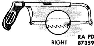
Do not apply too great or insufficient pressure to blade. Either abuse ruins blades. Apply just enough pressure on face stroke to make teeth "bite."
