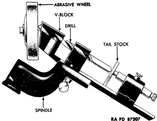
Inspect drill point to see if it has been ground back far enough to eliminate all nicks. Repeat grinding and inspection operations until perfect appearing points are obtained.
