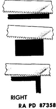
Do not install blade so teeth point toward handle. Blade will not cut properly. Point teeth away from handle, tighten securely, and retighten after first few strokes.
