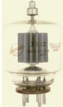
The reconditioning of a 3-500Z is relatively simple. With a DC voltage 0 - 40 V you should be able to get around 400 mA anode current with maximum 40 V DC on the anode. Apply 4.9 V to the filament and "cook" the tube for an hour. Then connect the variable supply and adjust DC for 400 mA anode current. The process must be maintained until for example a stable 38 V/400 mA is obtained.
