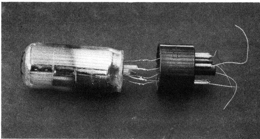
**Fig.3:** This 6X5GT/EZ35 has had the leads extended and inserted into the base pins ready for re-gluing. A 5-pin base would have converted it into a type 84, or with a side-contact type P base it would have become a replacement for a type EZ2.
