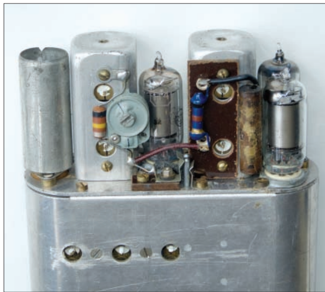
Fig. 6: The four valves and the b.f.o. switch (the two contacts and the metal shaft to the right of the centre valve).
