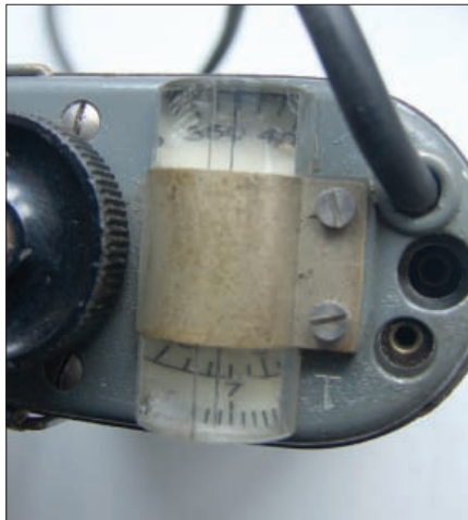
Fig. 4: The three tuning scales.
