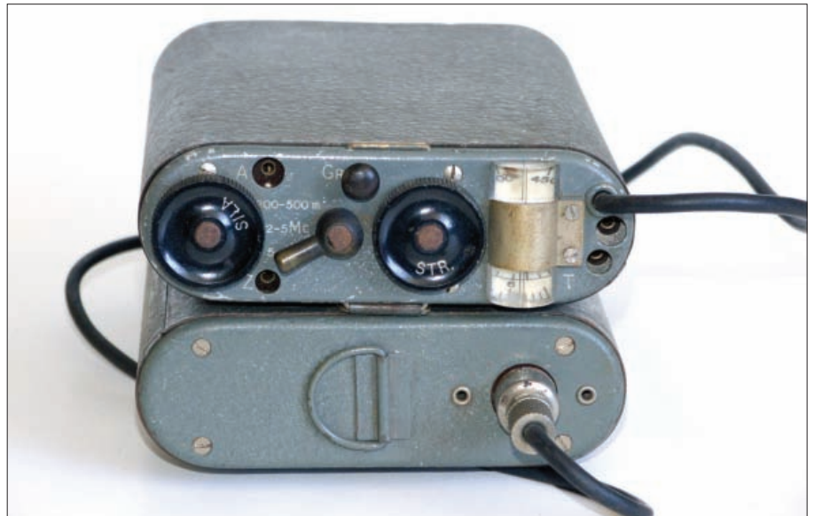
Fig. 3: The Polish OP3 receiver and battery box.
