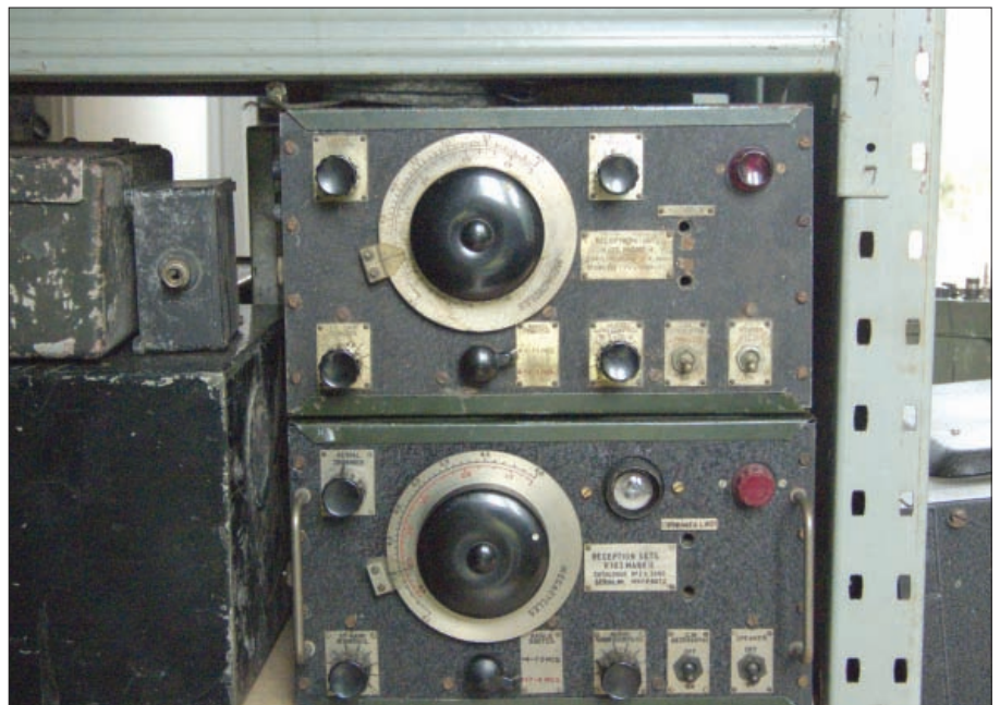
Fig. 2: The two R-103 receivers, note the 'magic eye' tuning indicator on the lower set.
