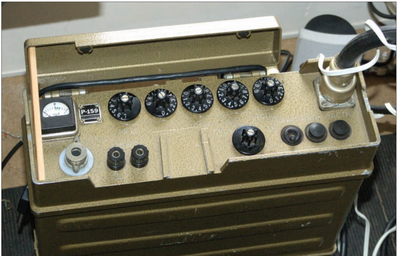
Fig. 1: The tuning controls of the R-159 transceiver.
