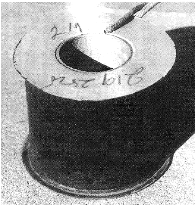
This 2.5kΩ field coil is wound on a cardboard former. Sealing the cardboard with lacquer will help to moisture-proof it.
