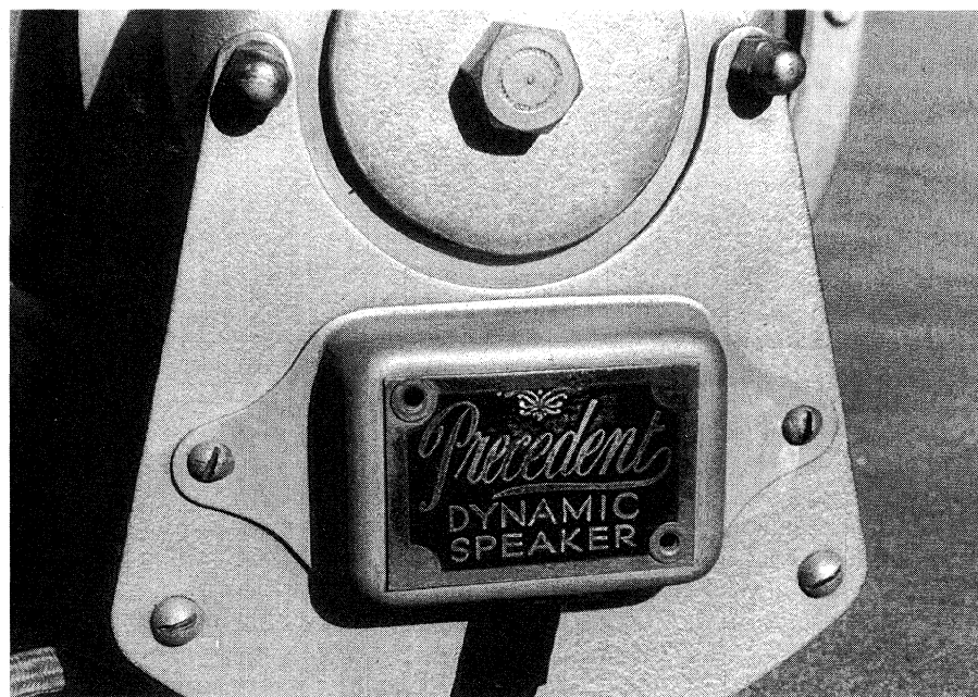
The large bolt head on this Precedent loudspeaker at top holds the central pole piece in place, making it easy to remove for repairs.
