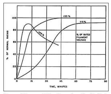
Summary of data accumulated by author on rejuvenation of thoriated tungsten filaments. Best results are obtained at 135% of rated filament voltage. At 115%, rejuvenation time is very significantly increased; at 165%, the tube is quickly destroyed.
