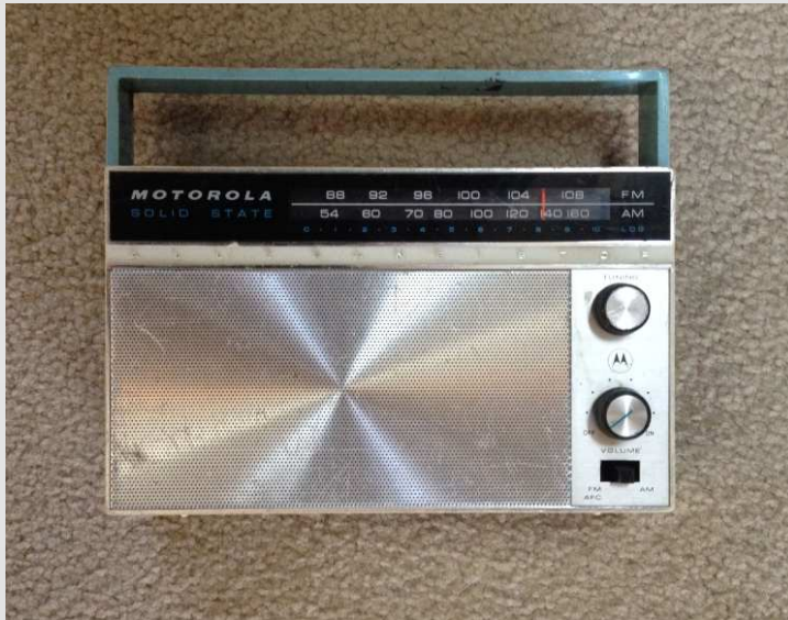
Portable AM Radio with internal ferrite bar antenna (sharp signal null off both ends)
