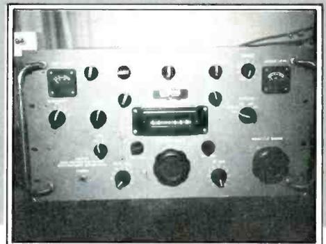
**AN/GRC-50.** Transportable FM set for two-way communications in the UHF range. Major components are the T-893 and R-1331.
