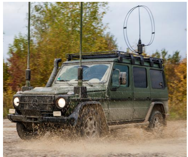
Figure 14 - Vehicle mounted loop antenna
