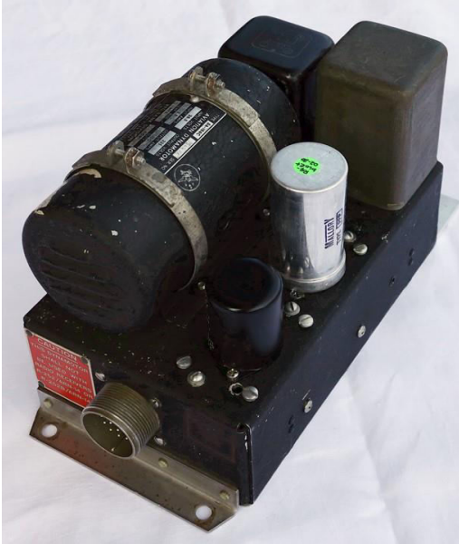
Figure 8. Dynamotor, topside (refurbished unit)
