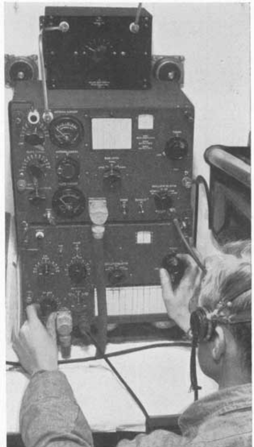
Model TCS transmitting-receiving equipment set up for operation. The antenna loading coil is mounted on top of the transmitter.
