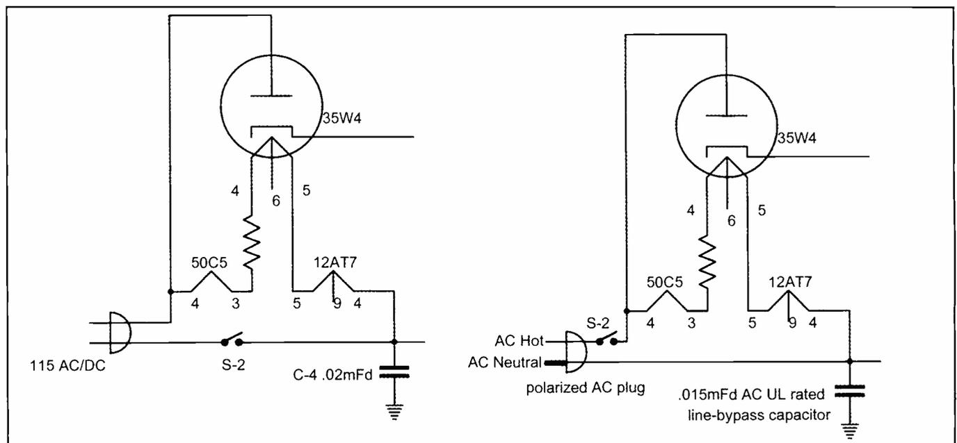
Figure 3: Here are the AC wiring changes.
