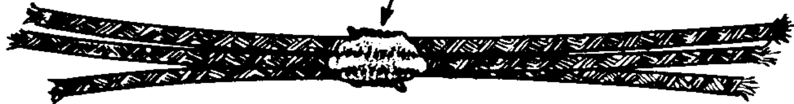
FIGURE 8. GROUNDING SHIELDED WIRES
