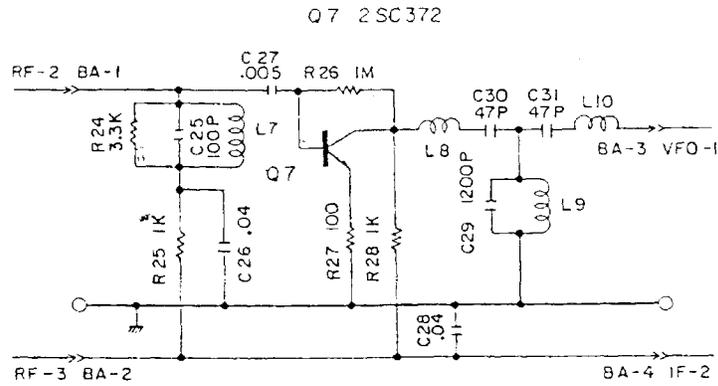
SCHEMATIC DIAGRAM OF BUFFER AMP
