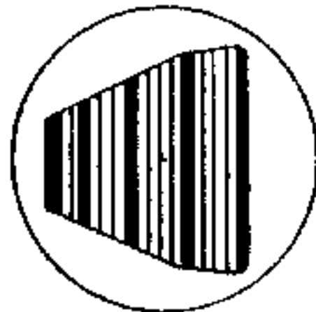
AM - Excessive Carrier Plus Flat Topping REDUCE CARRIER AND RETARD POWER OUTPUT CONTROL
