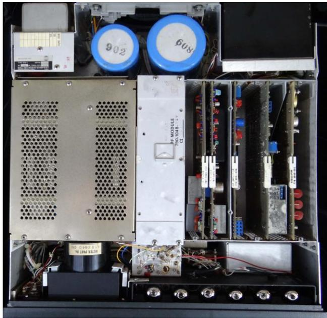
**Figure 4 - Card Rack with One Cover Off**
