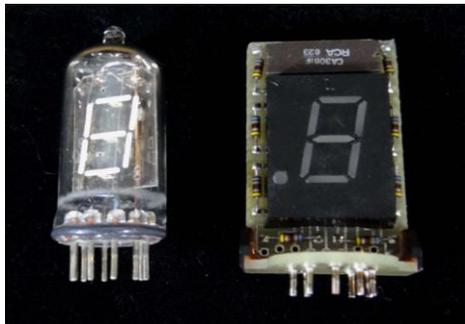
Figure 2 - VFD and LED Module
