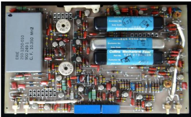
Figure 9 - IF Mechanical Filter Board
