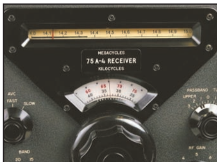
Figure 4—View of the Collins 75A-4 analog dial. Note that readout can be accomplished to the nearest 1 kHz—14,133 kHz in this example, a formidable achievement for 1955!
