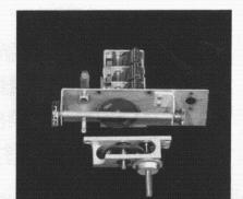
A rugged, solid 3/16" thick aluminum extrusion forms the backbone of the DR-30. This design technique (a DAVCO "first" in amateur radio design) is the basis for the extreme, rock-like stability of the DR-30.
