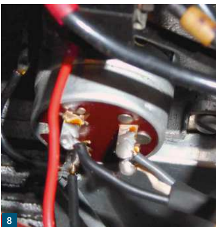
Fig. 6: The two Eddystone 840As. Fig. 7: Non-polarised power inlet on the 840A. Figs 8 & 9: The two different power switch connections. Fig. 10: Rubber power connector. Fig. 11: IEC C6 connector fitted. Fig. 12: IEC connector offered up to rear panel.
