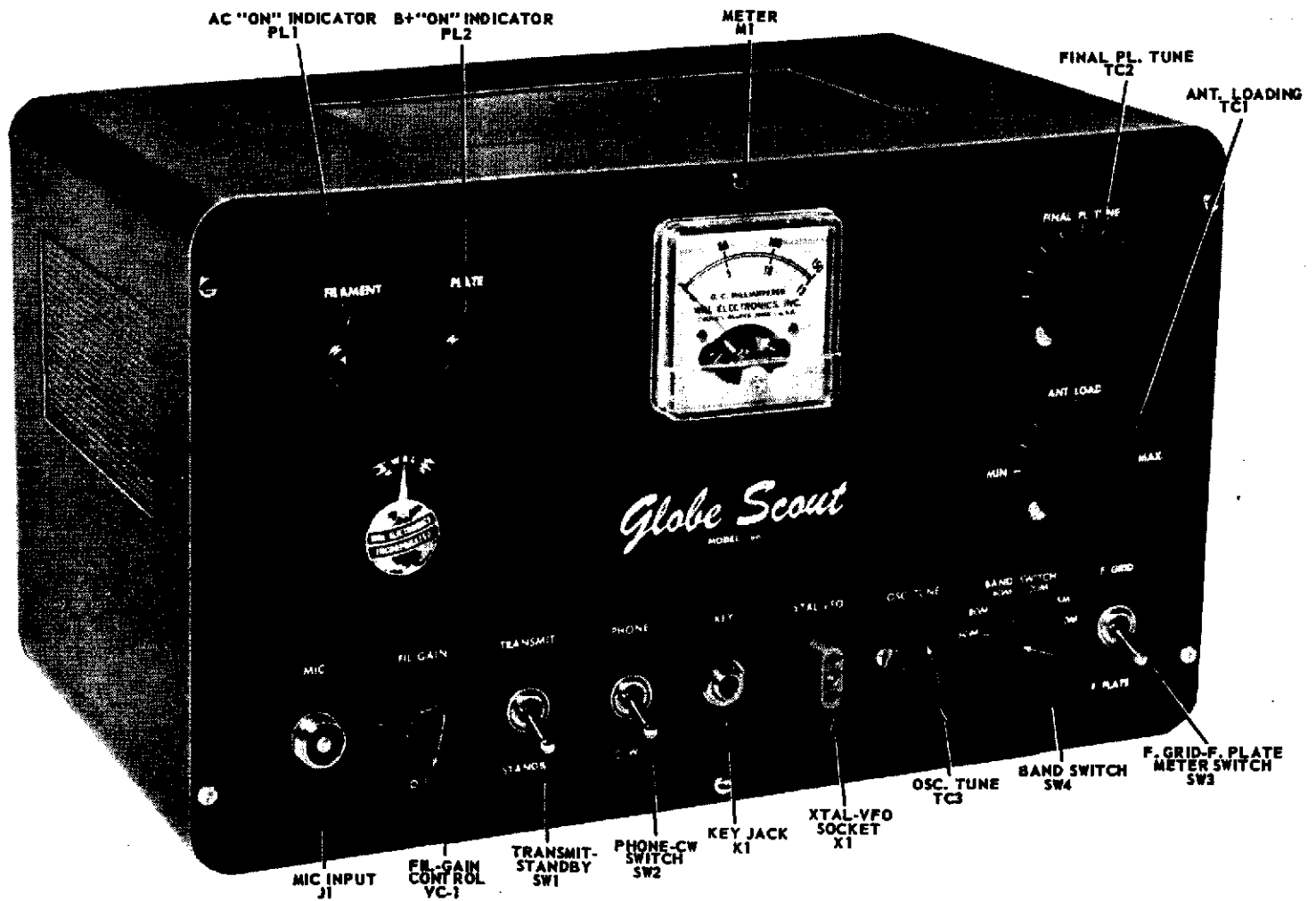
Figure 2. Panel Controls of Globe Scout Model 66.
