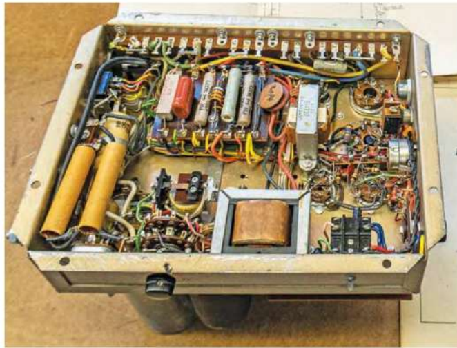
The transmitter power supply and modulator chassis.
