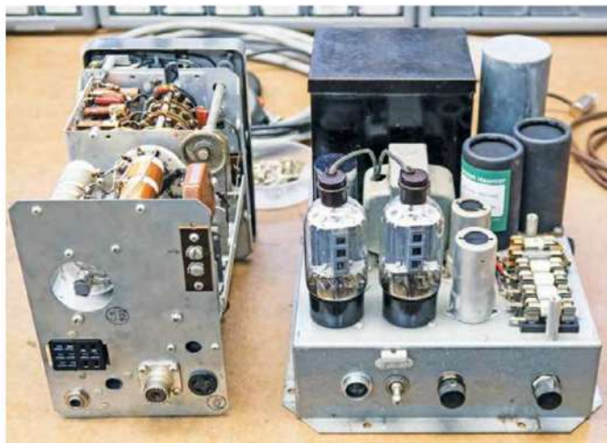
The transmitter and power supply uncased.
