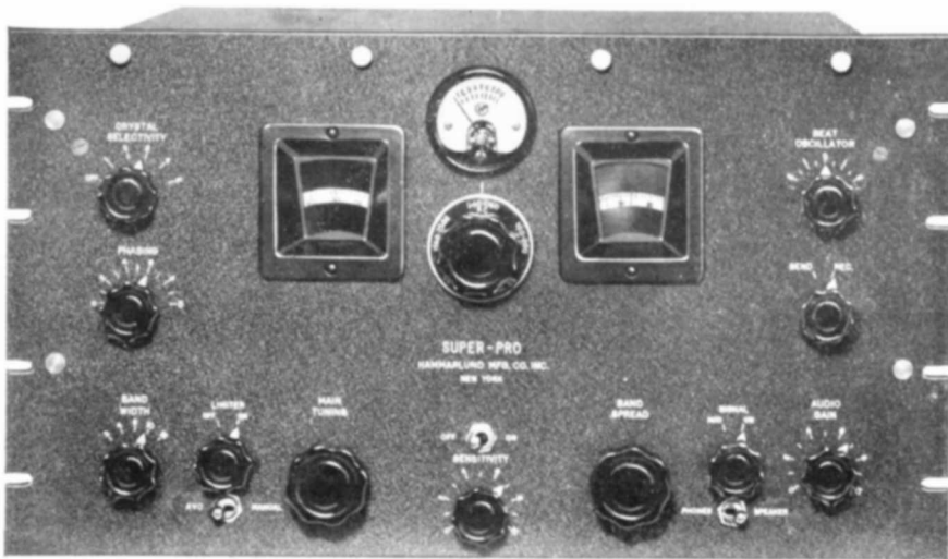
FIG. 8—"SPR-200-X", rack model, designed to fit standard 19" relay rack, complete with dust cover
