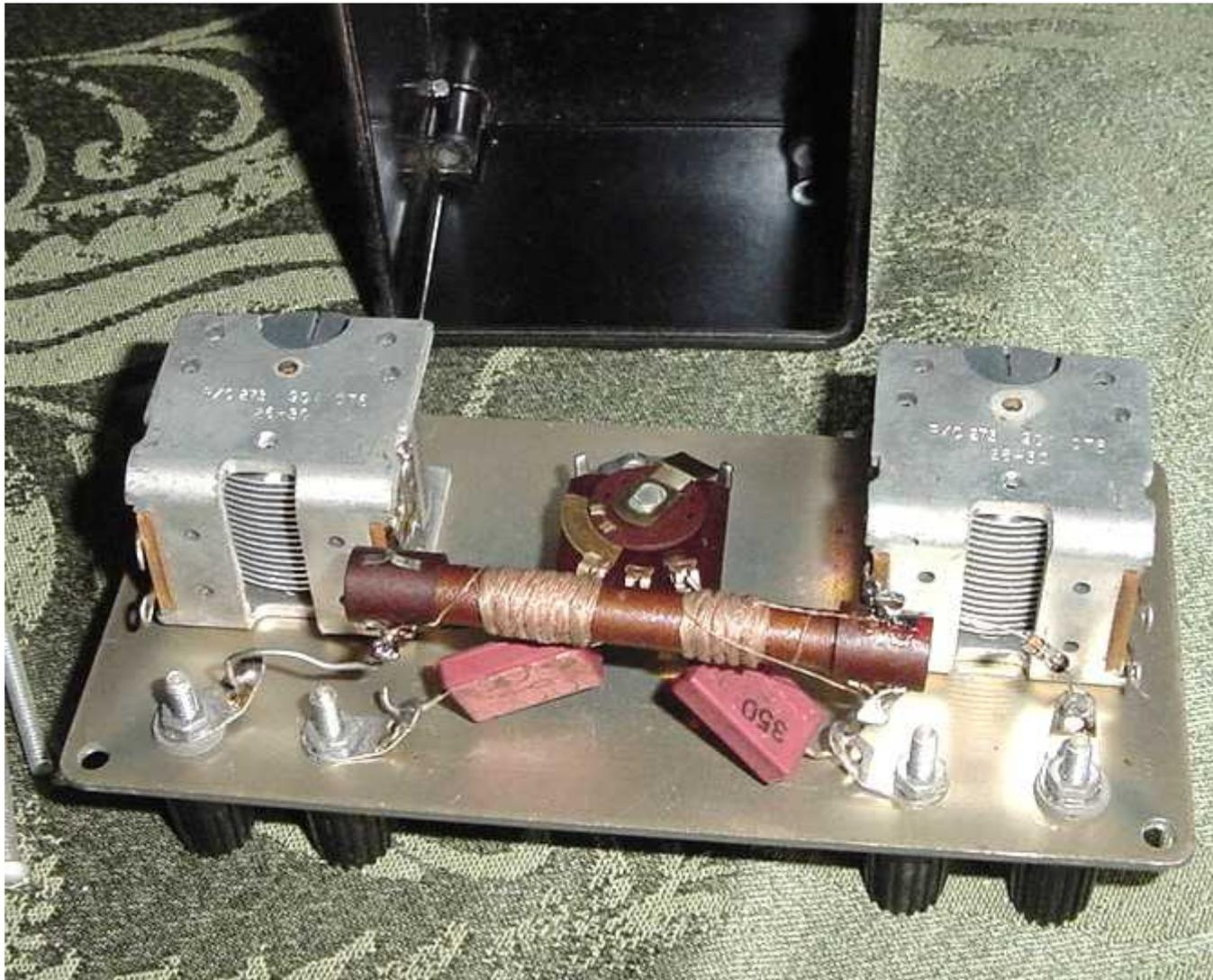
Another photo showing the inside of the original Heathkit CR-1. Note the rectangular pinkish mica capacitors, the configuration of the central antenna switch, the "cable knit" appearance of the coil windings, and the long screws holding the panel to the threaded stubs that are recessed deep into the cabinet.
