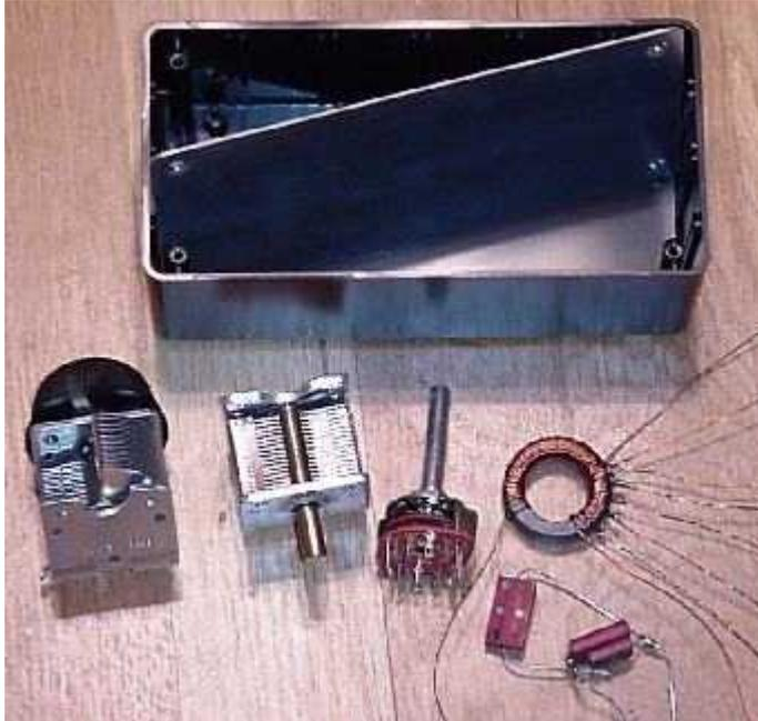
Here is a shot of the main parts on the floor. The rotary switch, diode, and box are from Radio Shack. The variable caps were obtained from the Xtal Set Society. The coil is described above and I got the old mica capacitors from my junk box. I ended up using a different coil and no padder capacitors though.
