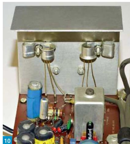
Unlike the GC-1A, which has a momentary action dial lamp switch when battery power is in use, the UK Mohican has a normal on/off type. The original dial lamps are rated 6.3V 110mA. They are connected in series with a 12Ω resistor and this chain draws about 100mA from a 12V supply, more than the quiescent current drain of the receiver itself. This can be greatly reduced by replacing the lamps by a pair of LEDs with an appropriately larger value of series resistor.
