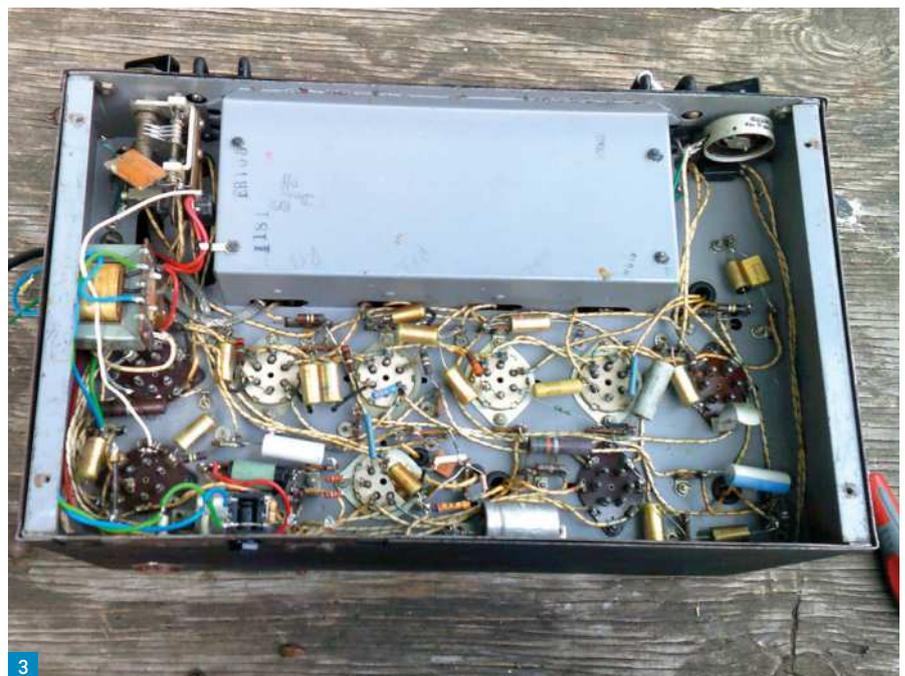
which intrinsically changes as the L/C (inductance/capacitance) ratio changes, a high-inductance primary is used in the inter-valve RF transformers, leading to the opposite, which is then compensated for by having a small top-coupling capacitor between primary and secondary. This however is not shown on the circuit diagrams.
