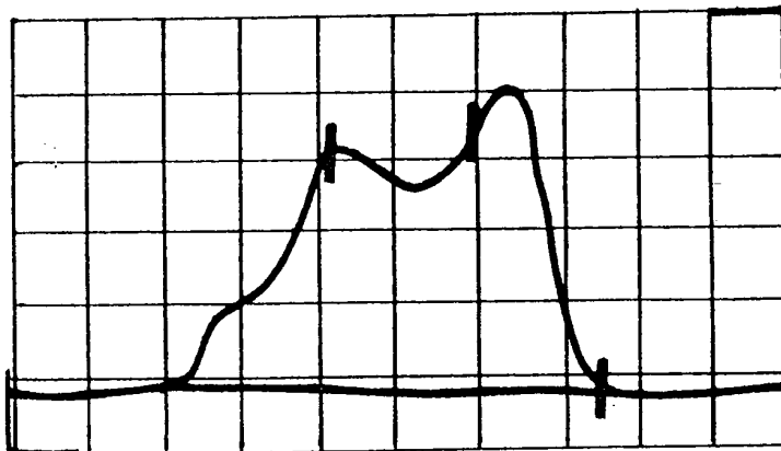
Fig. 18: MS-2 High Band Sweep (50 db attenuation -- (0.1 mv pp)
