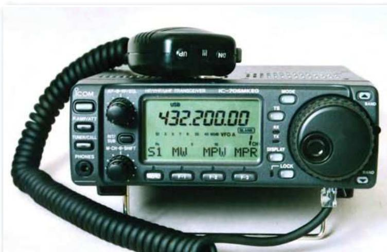
**Fig. 5:** The IC-706MkII G offered operation on the major Amateur bands from h.f. to u.h.f.
