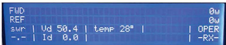
Figure 1 — The ANAN-8000DLE LCD shows forward and reflected power, SWR, drain voltage and current, temperature, and status (RX for receive).
