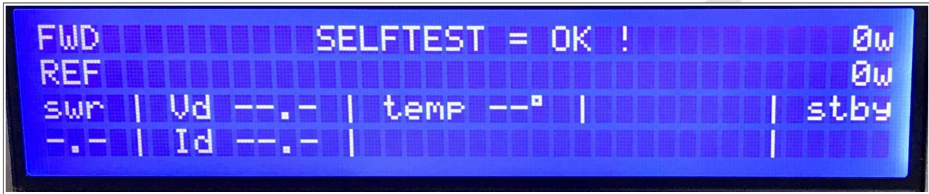
Self Test complete and all tested circuits working properly
