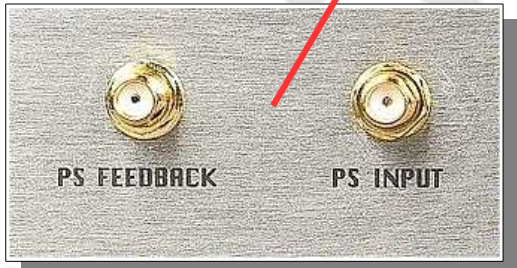
PureSignal connectors (usually looped together at factory)
