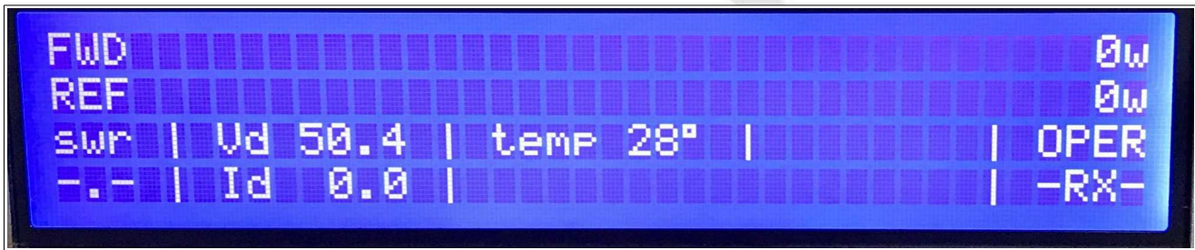
Operational LCD Display when ready for Rx and Tx
