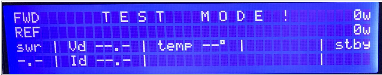
Self Test when power applied to the Transceiver
