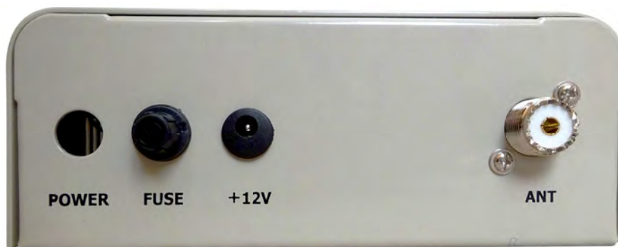
Fig. 3: The rear panel with the connectors and fuse installed. The hole labelled Power is for an alternative power supply for the PA stage (see text).
