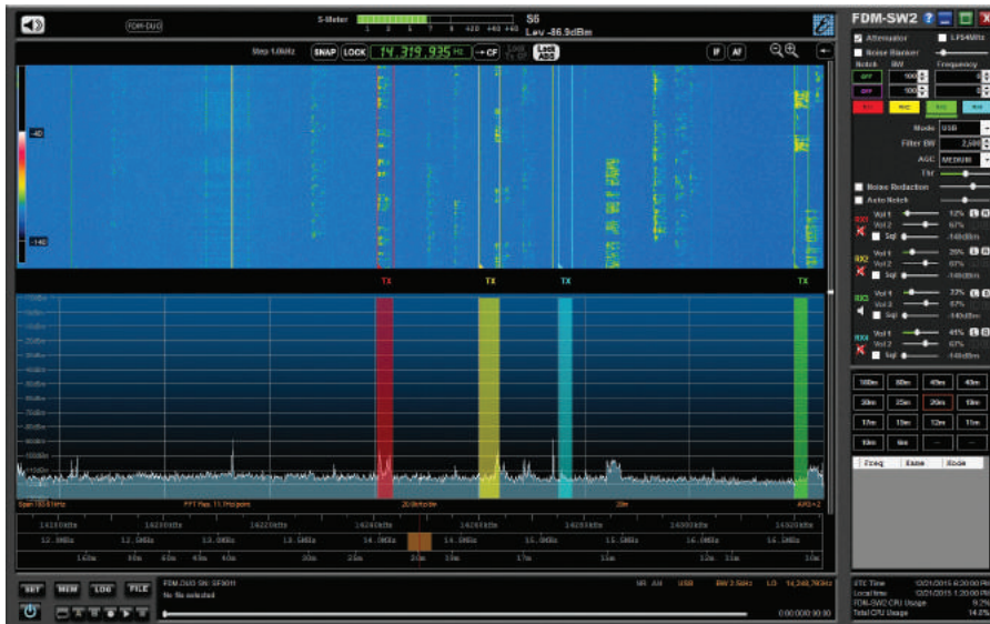
Figure 5 — The primary FDM-SW2 software display. Note the color-coded bars in the spectral display. Each one represents a separate receiver.
