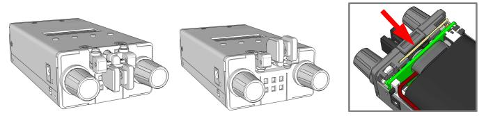
Contact spacing of the KHPD1 paddle can be adjusted using the hex wrench stored inside the enclosure (see arrow in the illustration above-right). Each paddle has a set screw in its housing. A fairly wide spacing is recommended for operation in high-vibration or less-stable operating positions.
