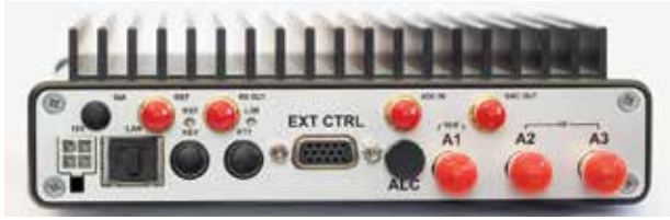
PHOTO 2: SunSDR2 PRO – rear panel connections.
