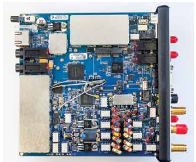
PHOTO 3: An inside view of the sunSDR2 PRO.
