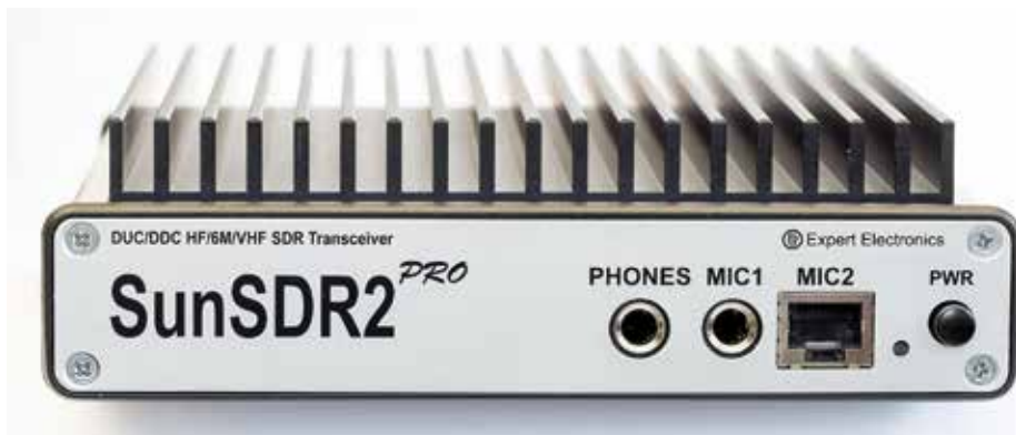
PHOTO 1: SunSDR2 PRO – front panel connections.
