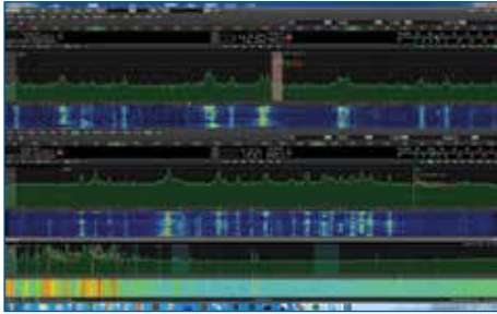
PHOTO 4: ExpertSDR2 software showing both receiver channels and the band-scope.
