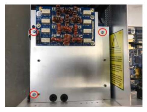
**Step 7:** Install a 4<sup>th</sup> screw included in the kit through the backside of the radio as shown below. It secures the mounting platform corner without a standoff.
