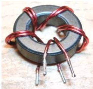
Picture 3, tinned wires
