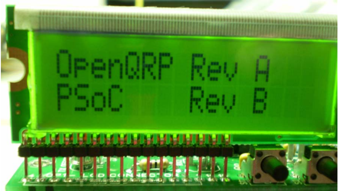
Here's the LCD sign on display with the PsoC IC installed. Note that the firmware revisions for both the main CPU and the PsoC are shown, the current revision will be different than these. Backlight can be turned on and off by a selection in the configuration menu.
