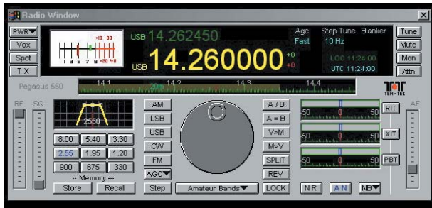
Top: The 'virtual transceiver' on the monitor when the Jupiter is controlled from a PC.
