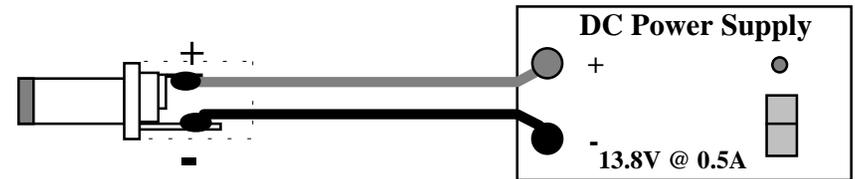
**Important Note:** In case of accidental reverse-power connection, your kit is protected against major damage by a "crowbar" diode (D1). However, activation will blow a "trace fuse" etched onto the circuit board next to the power connector. This must be replaced by a thin wire or a pig-tail type fuse before your kit will operate again (see "In Case of Difficulty").
