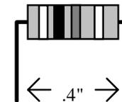
When installing resistors, save a few of the clipped-off lead ends--you'll need these for pc board jumpers later on.
