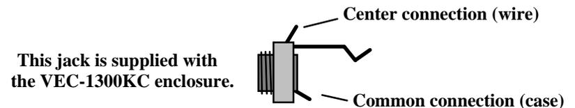
16. Identify the free end of the "key" hook-up wire. Connect to the center-connection terminal of one 1/4" jack.
