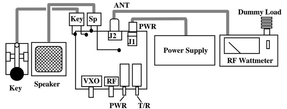
To test the radio outside of a metal case, you'll need to install temporary "ground" or "common" leads for the key and speaker jacks. Use temporary lengths of hookup wire or clipleads to make these connections. These may be attached to any convenient point on the pc board ground surface.
