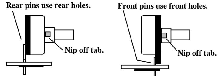
12. Install the 1K potentiometer at R1 and solder.
