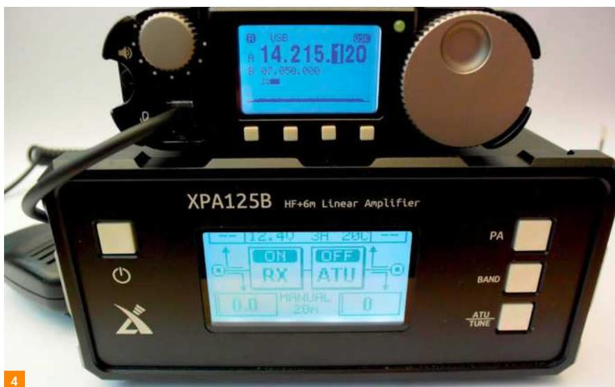
interconnecting leads, it becomes a simple plug-and-play operation to connect a computer and/or the XPA-125B linear amplifier. The handbook recommends the installation of a CH342 port driver and use of the same datcomms software as per their G90 radio.
