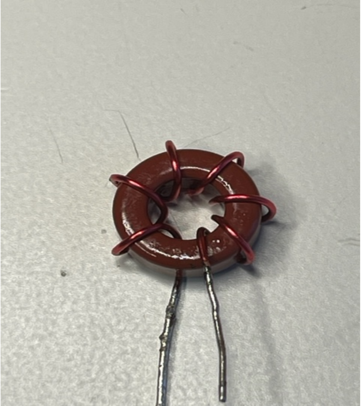
This is T37-2 RED Toroid with 7 turns of enameled copper wire.
