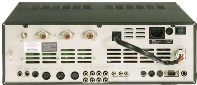
Figure 5 — Jacks on the FT-2000's rear panel are easy to get to and well marked.
