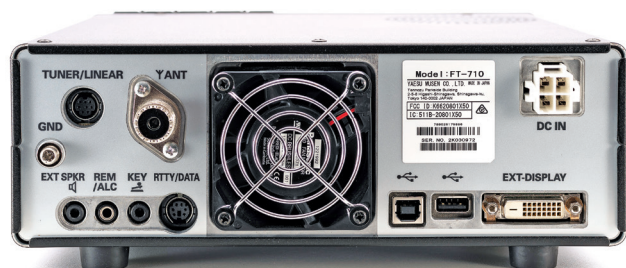
Figure 1 — The FT-710 rear panel.
