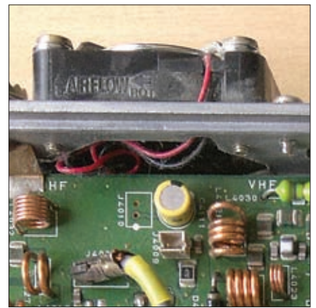
The real panel fan disconnected from J4009.
