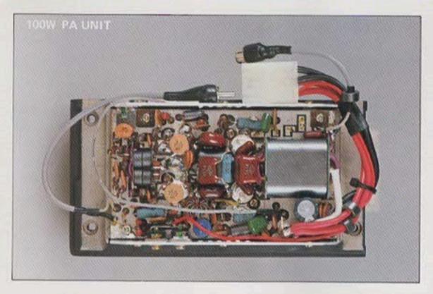
Rugged power transistors with extensive protection circuitry are your assurance of reliable operation for many years to come. Completely broadbanded, the FT-ONE transmitter requires no tuning for instant operation on any band for which it is configured. Crossband full breakin operation is a prime example of the flexibility afforded by the broadband solid state design.
