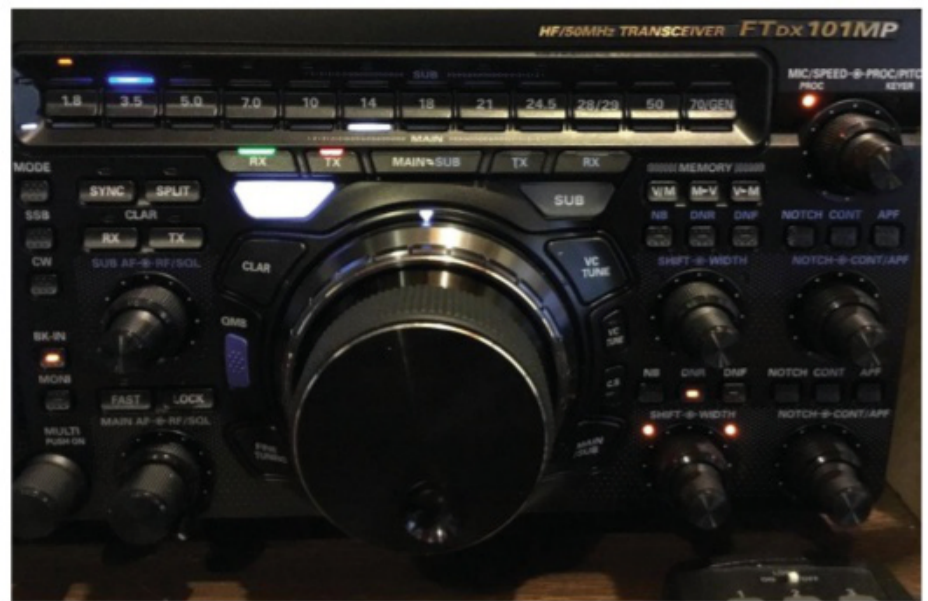
Photo E. The front panel shows the buttons around the MPVD ring (see text for details). Notice also the two identical sets of controls to the right of the MPVD. The top one controls the sub-receiver while the main receiver controls are on the bottom.
