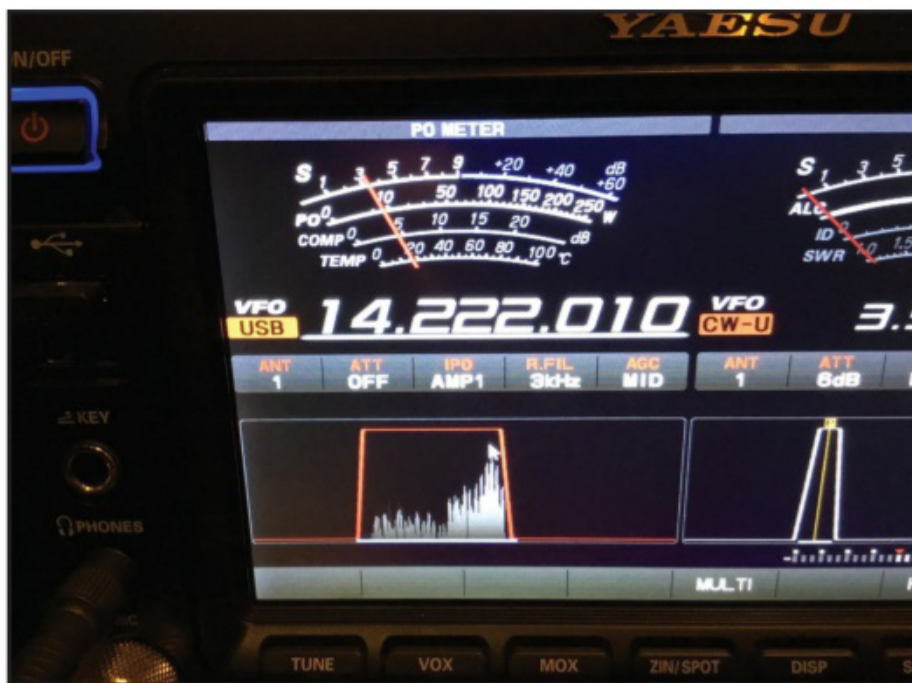
Photo C. While listening to A71FJ, a nearby SSB signal appeared within the receiver passband. The interfering signal is shown under the small arrow.
