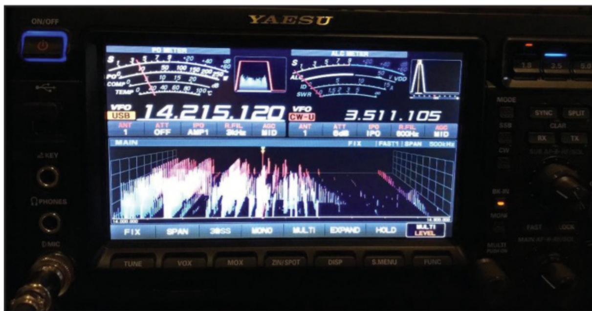
Photo B. The 3DSS screen on the FTdx101. It shows not only activity, but signal strength and time as it fades into the distance. (Photos B-E by the author)
