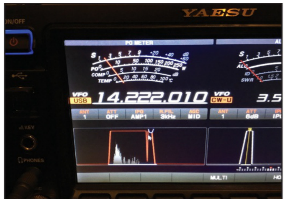
Photo D. By using the contour (small u-shaped image) and notch (long v-shaped image) controls, the interference is gone. The interfering station is still transmitting, as can be seen by turning the contour and notch controls on and off.
