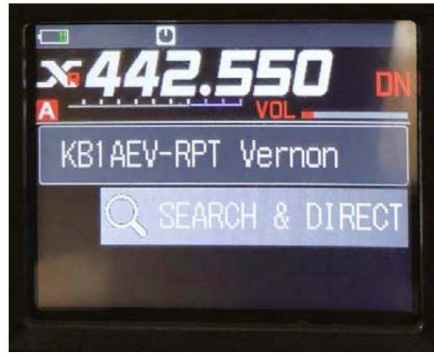
Figure 2 — Accessing the Yaesu WIRES-X network through the KB1AEV Fusion repeater.
