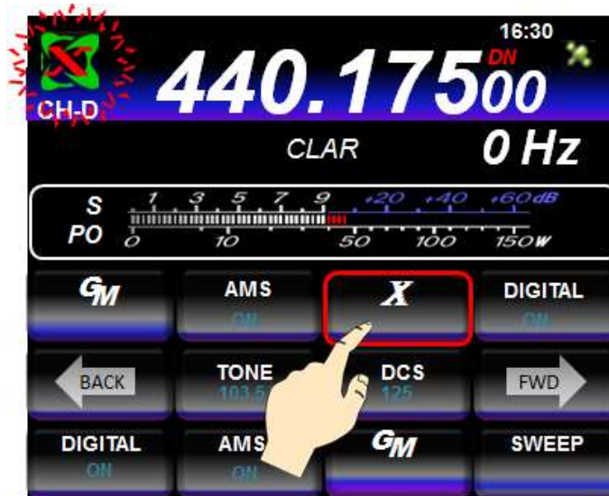
Figure 71 The FT-991 automatically switches to transmit mode and “X” and WIRES X icon flashes.
