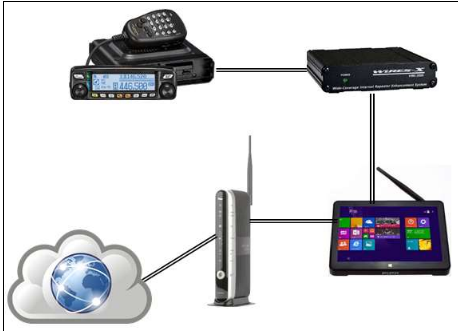
Figure 125 The WIRES X Local Node
