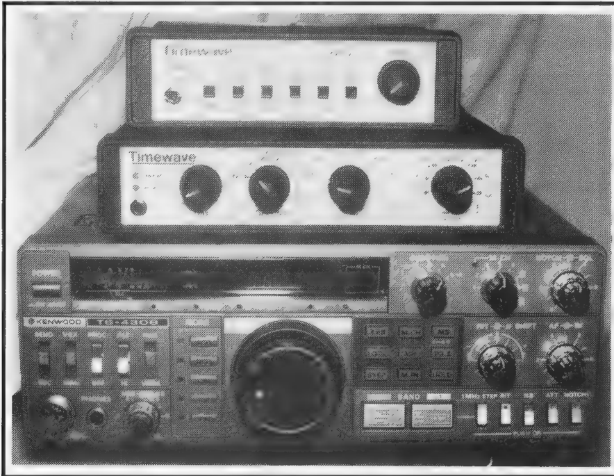
The DSP-9 and DSP-59 sitting on top of the Kenwood TS-430S transceiver used in the evaluation of the filters.
