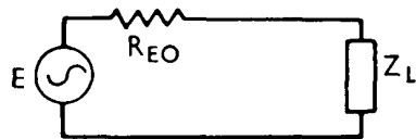
FIGURE 4 OUTPUT CONDITIONS USING SERIES RESISTOR
