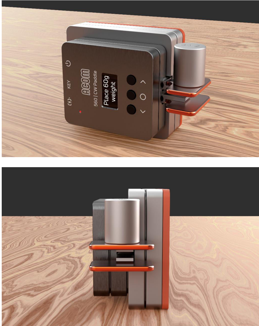
Figure 3-5 | Right lever with placed calibration weight
